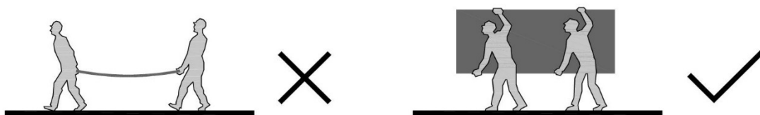
Figure 1.14 - Viroc panels Handling
