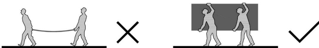
Figure 1.14 - Viroc panels Handling
